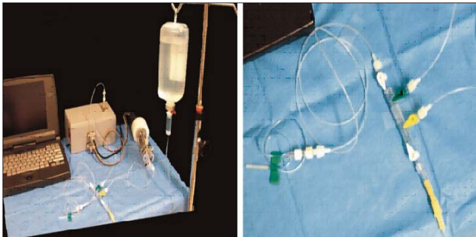
Figure 1. Ocular rigidity measurement device representation. The computer unit and transducer readout electronics, the mechanical dosage system (similar to an infusion pump) (left), and the saline tubing manifold (right).
